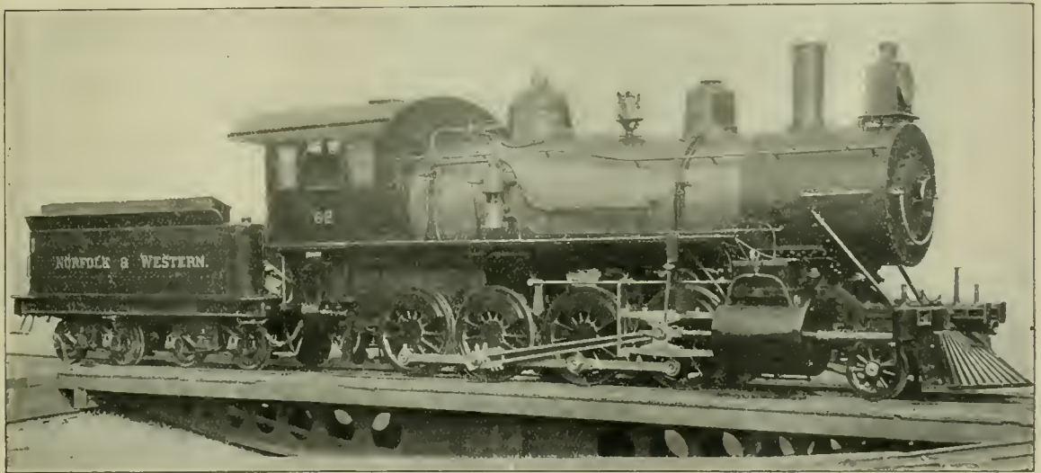
BALDWIN TWO CYLINDER COMPOUND.
